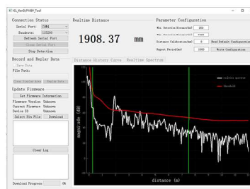
Liquid level and position detection demonstration tool Real-time display of distance history curves and detection waveforms
