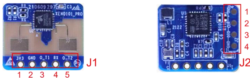
Figure 3-1 Top and bottom device map of XenD101Pro
