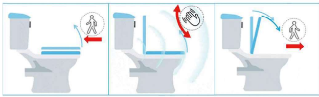
Open lid when approaching Open seat by gesture recognition Close lid and seat when leaving
