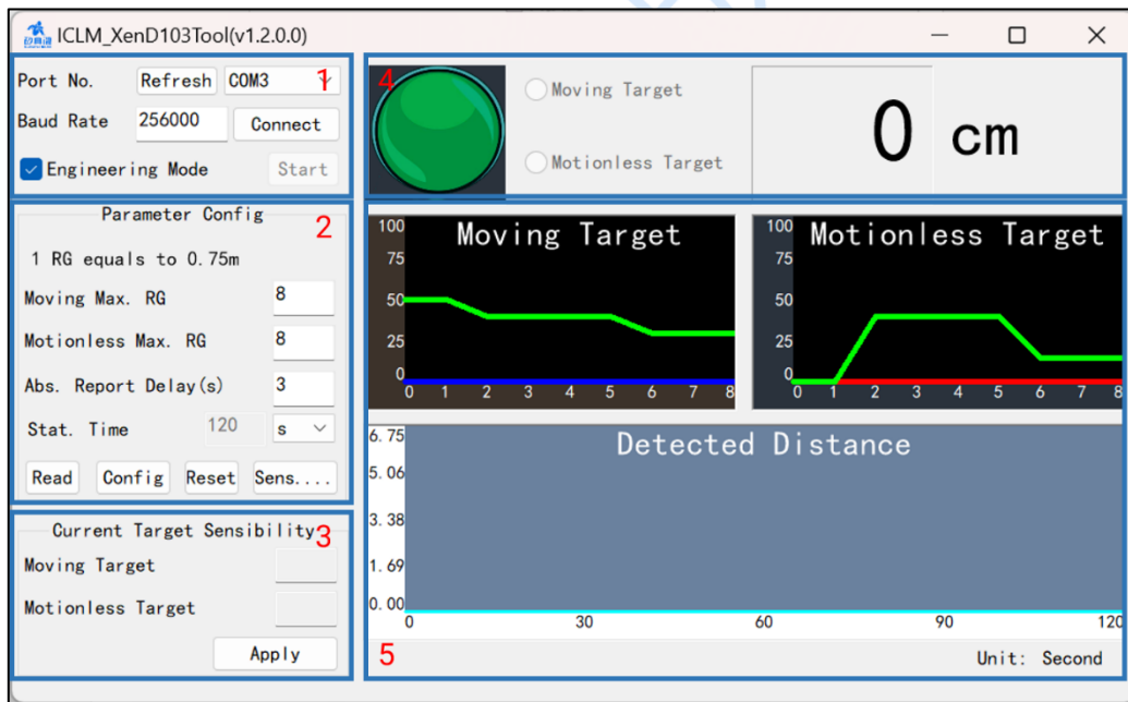
Figure 4-2 GUI of the ICLM_XenD103Tool
