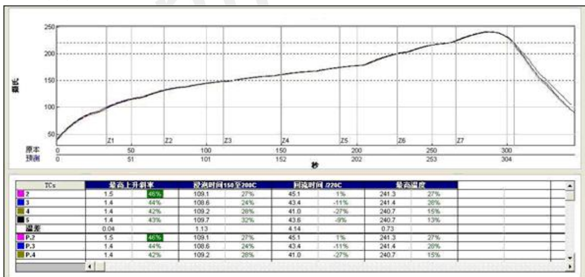
Figure 17: The Ramp-Soak-Spike reflow profile of SIM68AT
