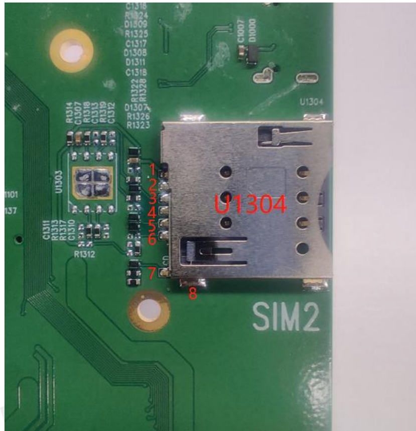
Figure 7: SIM card socket and its pin
