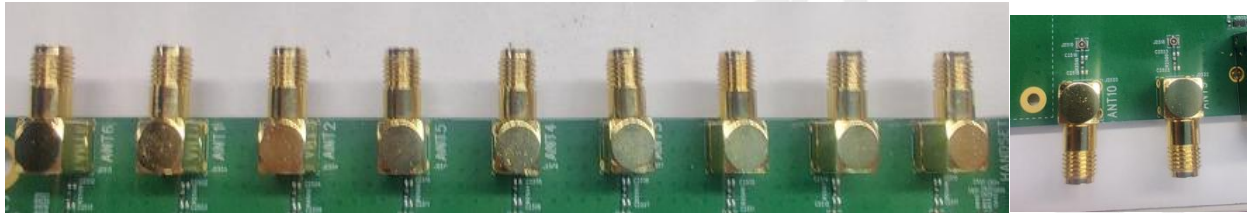
Figure 20: SMA antenna interface
