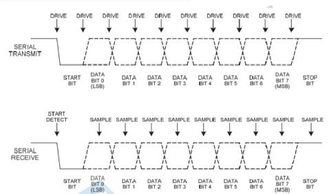
Figure 4: UART Interface Waveform PIN diagram
