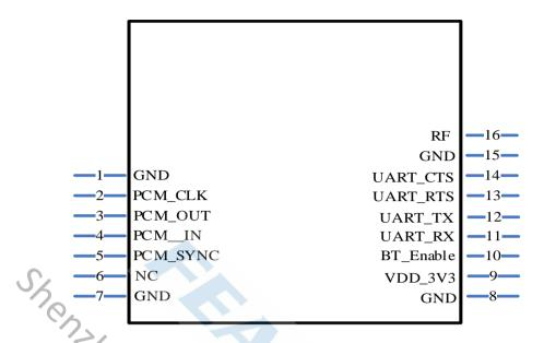
Figure 2: FSC-BT825B PIN Diagram
