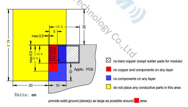
Figure 17: FSC-BT825B Restricted Area
