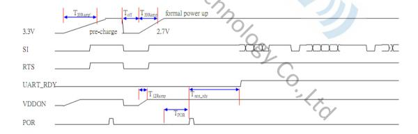
Figure 5: UART Power-On Sequence without Hardware Flow Control
