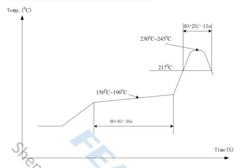
Figure 15 Typical Lead-free Re-flow Solder Profile
