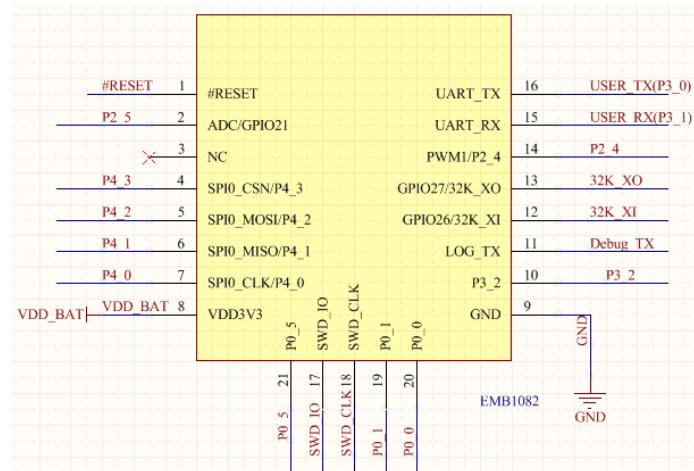
Figure 12 External Interface Circuit of EMB1082
