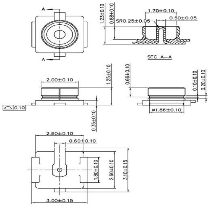
Figure 5 Size of External Antenna Connector
